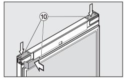
■ Refit the covers <sup>10</sup> onto the appliance door.
